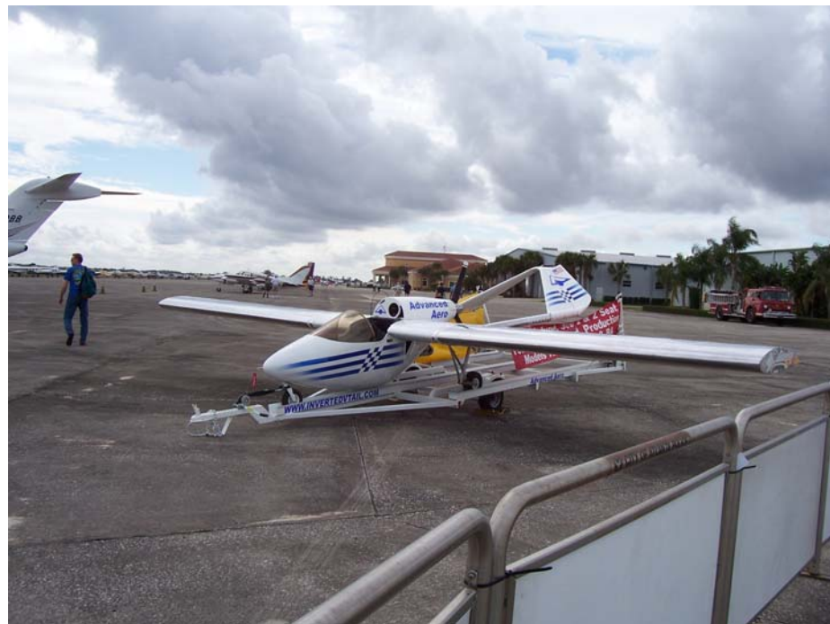
One of two inverted V-tail Light Sport Aircraft designs offered by Advanced Aero of Titusville, Florida
